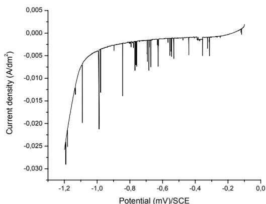
**Fig.1.** Polarization curve for described solution of electrolyte used for Zn-Co co-deposition recorded for the potential range from -100 mV to -1200 mV, 32°C temperature, with magnetic stirring of the electrolyte
