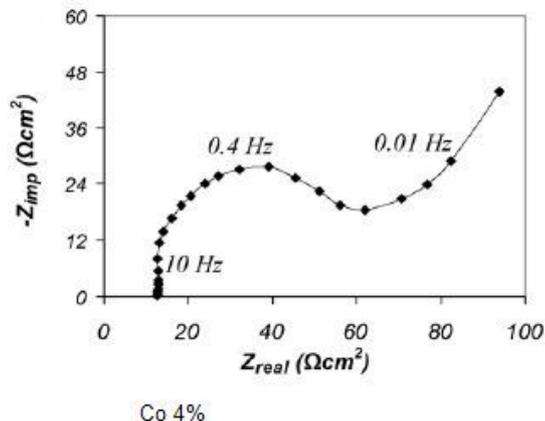
**Fig.4.** Nyquist impedance curve obtained for the first solution (higher concentration of Co ions)
