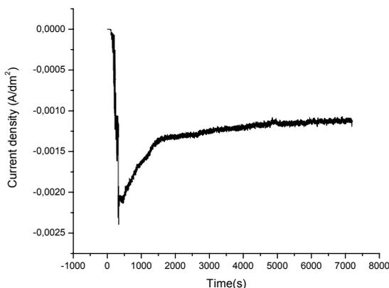
**Fig.2.** Crono-amperogramme recorded during Zn-Co alloy co-deposition at -1000 mV potential and 32°C, with magnetic stirring of the electrolyte
