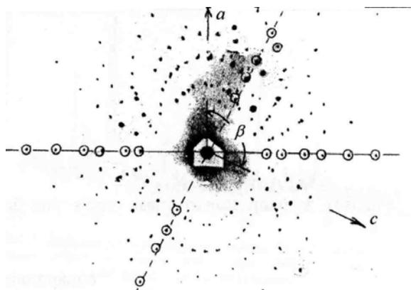
Fig. 3. Laue pattern of the single crystal obtained in the Pd-44.5 at. % alloy
