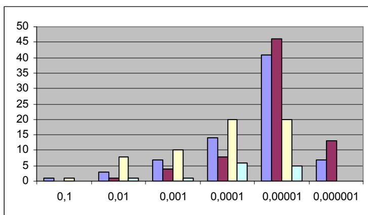
Fig. 1. Changes in the impurity distribution in lutetium after vacuum distillation. Blue, red, and white columns correspond to number of impurities (whose contents correspond to a level shown in the X-axis) in commercial Lu (wt %), distilled Lu (wt %), and distilled Lu (at %), respectively. Bluish columns indicate number of REMs (at %) in distilled Lu.
