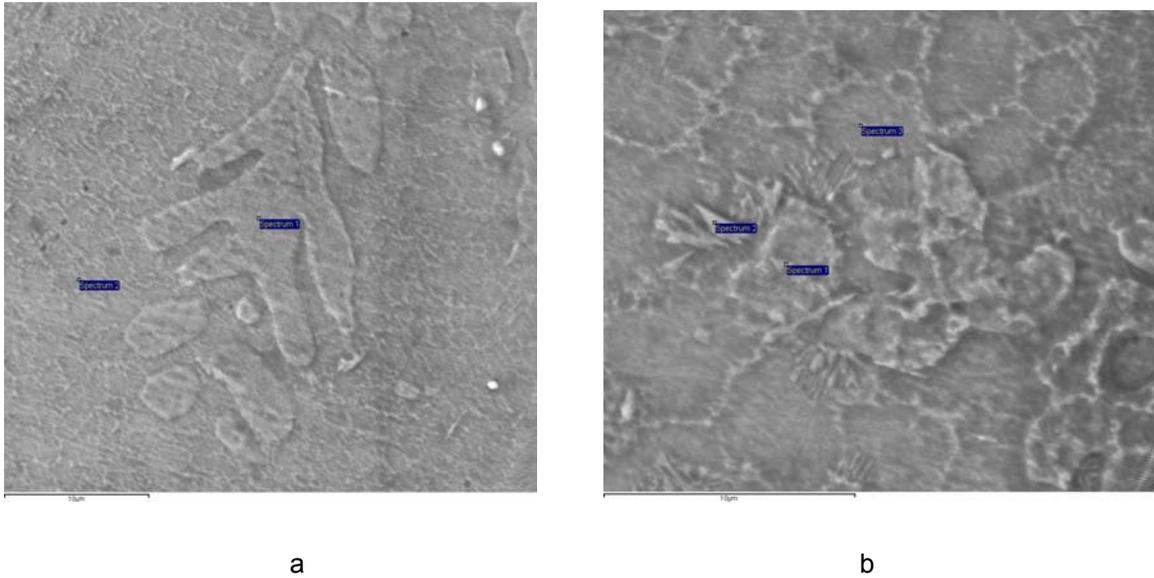
Fig. 4. Electron micrographs of the as-cast Pd-32.5 at. % Lu alloy.
