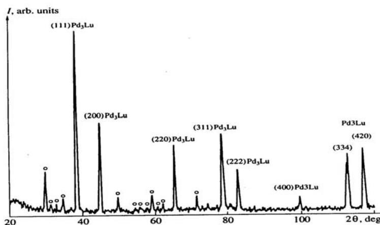
Fig. 2. X-ray diffraction pattern of the Pd-30 at. % Lu powder annealed at 1000°C for 100 h (Cu  $K_\alpha$  radiation).
