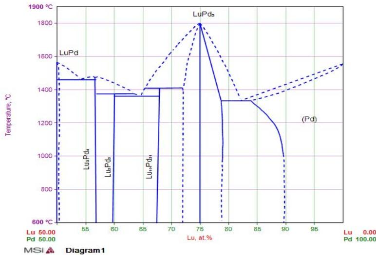
Fig. 5. Portion of the phase diagram of the Lu-Pd system.
