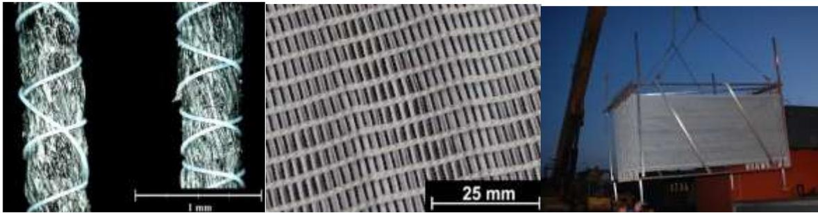
**Fig. 1.** a) A nanofibre thread with protective polyethylene fibres, b) woven planar structure of nanofibre bound threads and c) final carrier module.
