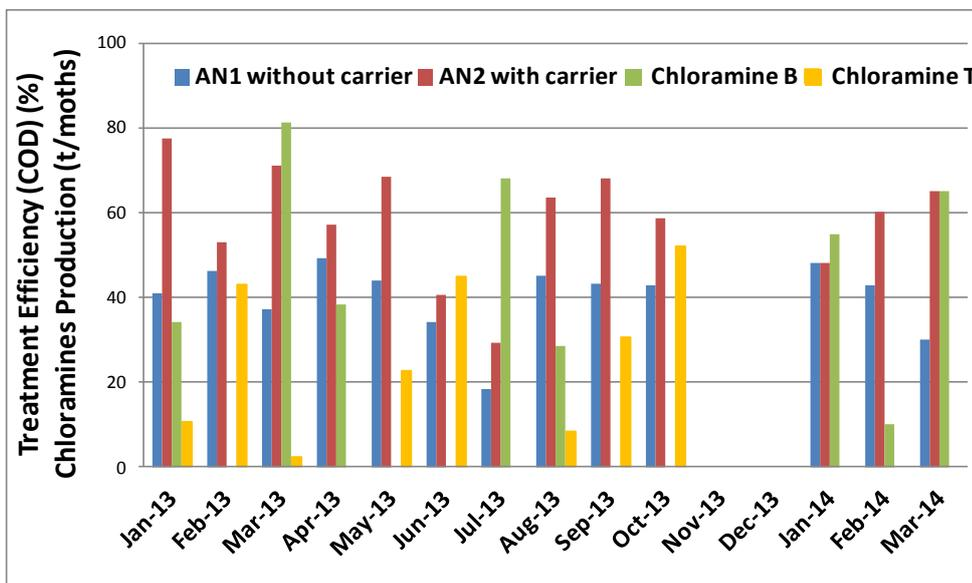
Fig. 3 Comparative study of both the conventional activated sludge system and the hybrid system with the nanofibre carrier
