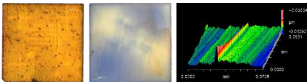
**Fig. 1** Optical microscopy picture of a boron doped diamond layer grown on a (100) oriented single crystal with a  $[\text{TMB}]/[\text{CH}_4]$  ratio of 500 ppm (left); Optical microscopy picture of as received Sumicrystal UP from Sumitomo Electric Hartmetall GmbH (middle); surface morphology measured by optical profiler (right).
