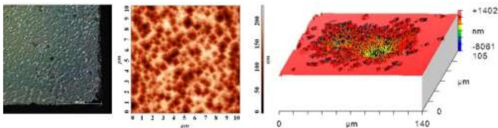
**Fig. 2** Optical microscopy pictures and (middle) AFM pictures of Ib (100) oriented single crystal after  $\text{O}_2\text{-H}_2$  plasma etching (left). Surface profile large pits formed during plasma etching measured using optical profiler (right).
