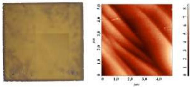
**Fig. 5** Optical microscopy image (left) and atomic force microscopy image (right) of boron doped epitaxial diamond layer (1000 ppm) deposited on re-polished sample and etched substrate.
