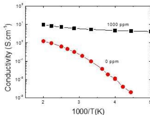
**Fig. 7** Arrhenius plot of conductivity of not intentionally boron doped diamond layers and doped (1000 ppm) boron doped diamond layers.
