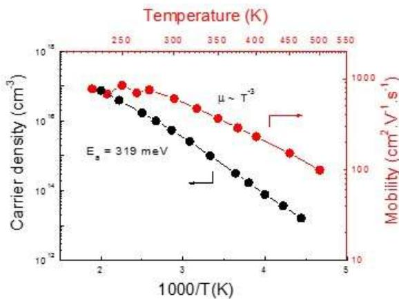
**Fig. 6** Arrhenius plot of carrier concentration and log-log plot of Hall mobility as a function of temperature of not intentionally boron doped diamond layers.
