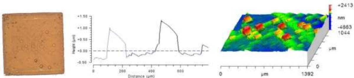
**Fig. 3** Optical microscopy picture of a boron doped diamond (1000 ppm) layer grown on 7 hours etched (100) oriented single crystal (left); 1D (middle) and 3D (right) surface profile of boron doped diamond layer's surface measured by optical profiler.
