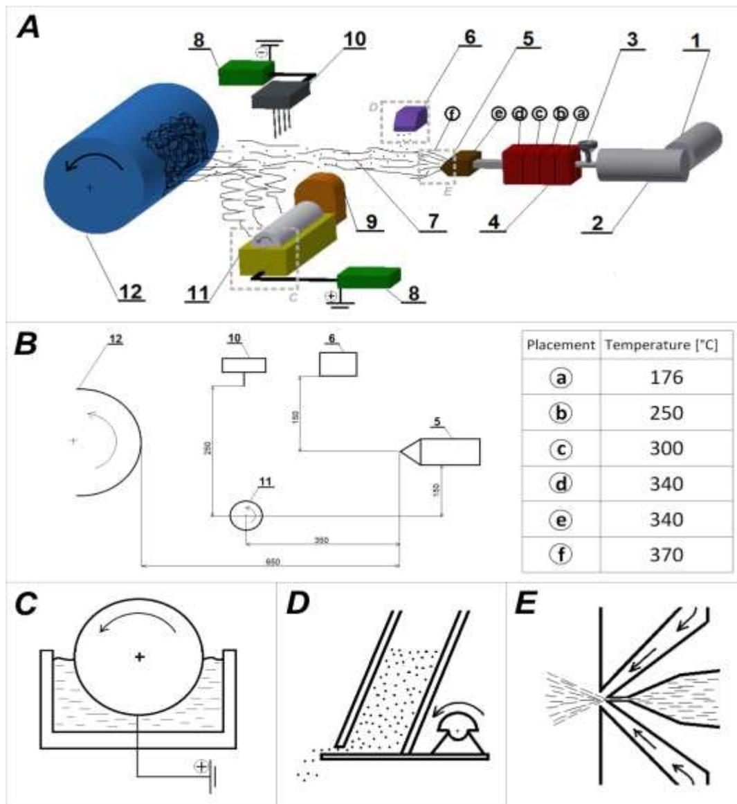
Fig.1. Scheme of the combination of meltblown and electrospinning with integration of particles in-situ into the producing fibrous material: scheme of all set-up (A); proportion description in millimeters and optimal temperature set-up (B); details of needle-less electrospinning spinning electrode (C), sputtering device (D) and meltblown die (E) set-ups.
