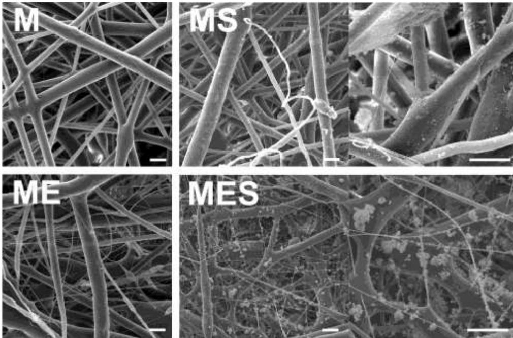
Fig. 2: Scaffold morphology observed by SEM for all four tested materials, scale bar is 20  $\mu$ m.
