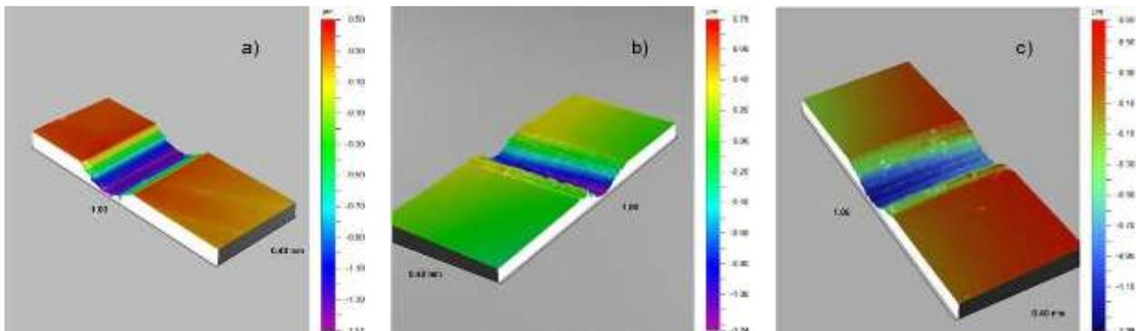
Fig. 7 3D Profile of PF 1 after tribology: a) clean solution; b) 0,3g/l AgNO<sub>3</sub>; c) 0,3g/l AgNO<sub>3</sub>+0,1g/l C<sub>6</sub>H<sub>8</sub>O<sub>6</sub>
