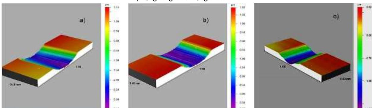
Fig. 8 3D Profile of PF 2 after tribology: a) clean solution; b) 0,3g/l AgNO<sub>3</sub>; c) 0,3g/l AgNO<sub>3</sub>+0,1g/l C<sub>6</sub>H<sub>8</sub>O<sub>6</sub>
