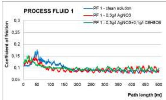
Fig. 5 Coefficient of friction PF 1
