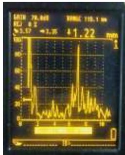
Fig. 2: Without defect.
