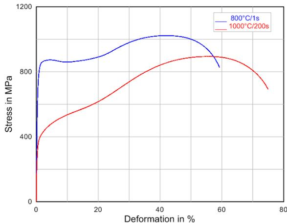
**Fig. 2** Stress-strain curves obtained from tensile test for 301LN steel annealed at 800 °C/1 s and 1000 °C/200 s
