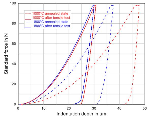
**Fig. 3** HV10 loading curves of material before and after tensile tests for 301LN steel annealed at 1000 °C/200 s and 800 °C/1 s
