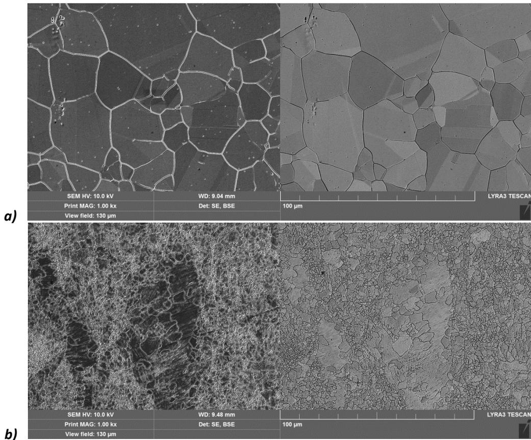
**Fig. 1** SEM micrograph in SE (left) and BSE (right) mode of the austenitic stainless steel 301 LN in non-deformed state (a) coarse grained structure after annealing at 1000 °C/200 s, (b) ultrafine grained material annealed at 800 °C/1 s
