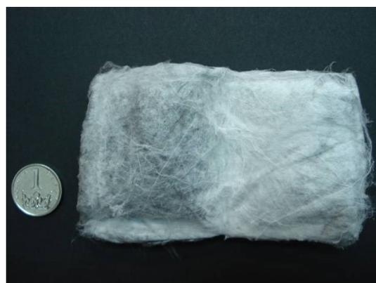
**Fig.2** Surface and dimension of composite nanofibrous material 50x100 mm (Diameter of Czech crown is 20mm)
