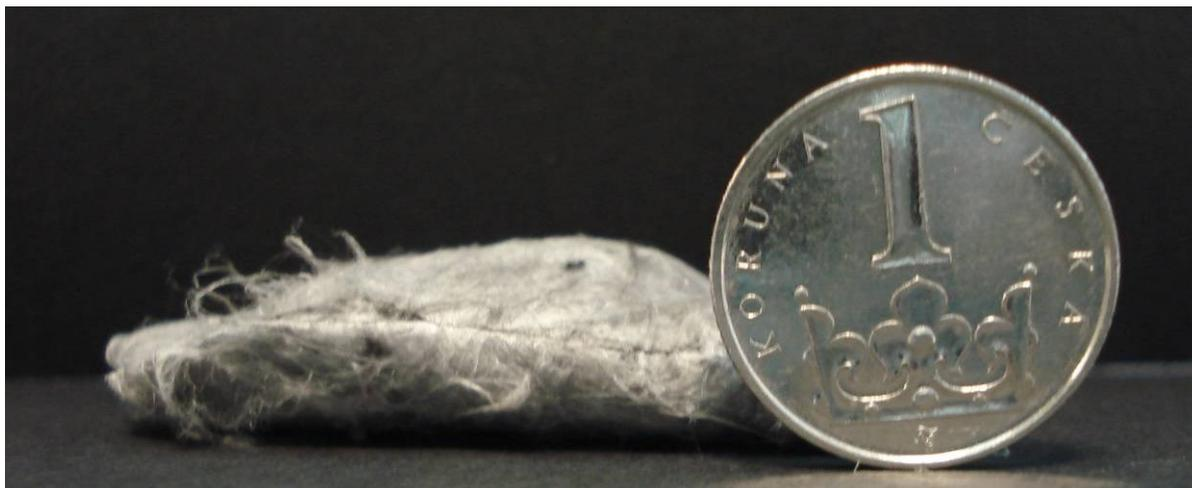
**Fig.3** Cross section of voluminous nanofibers composite material, the thickness 10mm (Diameter of Czech crown is 20mm).
