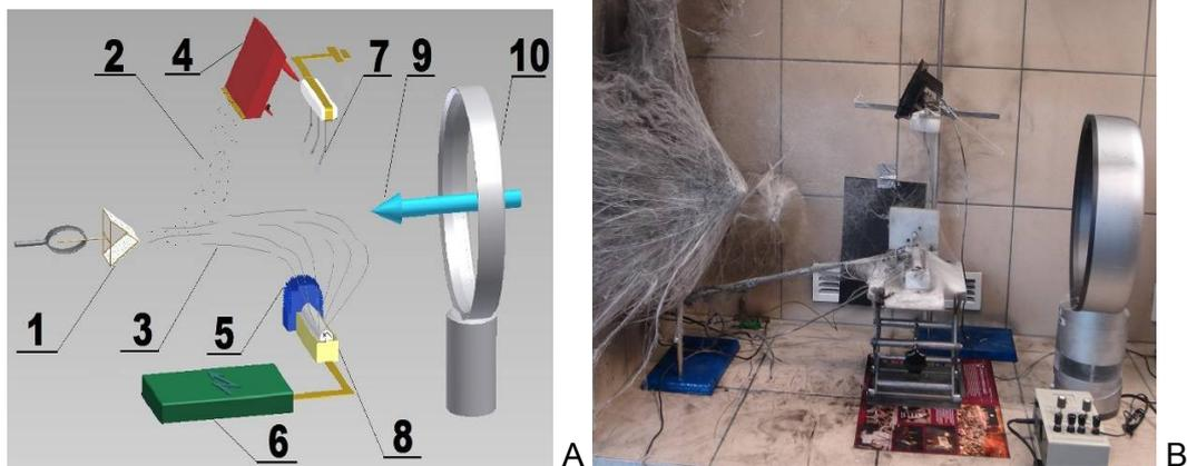
**Fig.1A** Schematic view of electrospinning equipment and air blowing equipment. 1-wooden frame in holder and deposited nanofibrous layer, 2-active carbon particles, 3-nanofibres, 4-box with active carbon and dosing apparatus, 5-engine connected with roller, 6-high voltage supply source, 7-grounded needle collector, 8-nanospider, 9-focused smooth air, 10-blade less air multiplier. Fig.1B: Experimental setup placed in the digester.
