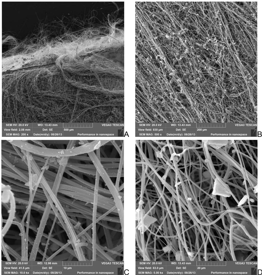
**Fig.4** A-SEM fluffy voluminous structure of PVB, B-SEM surface structure, C-SEM detail view to PVB nanofibers and particles, D-SEM detail view to nanofibers with incorporated active carbon particles.
