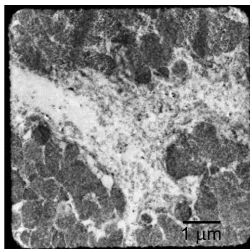
**Fig. 7.** Ultrathin section of mouse heart muscle prepared with no post-fixation or staining. STEM micrograph at 500 eV, bright-field image, beam current 13 pA.
