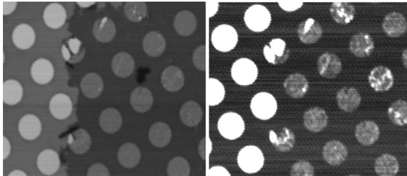
**Fig. 4.** A 3 nm gold film, prepared by magnetron sputtering and deposited on the Quantifoil; electron energy 3 keV (left) and 10 eV (right), the diameter of the holes in the supporting carbon foil is 2  $\mu\text{m}$  [9].
