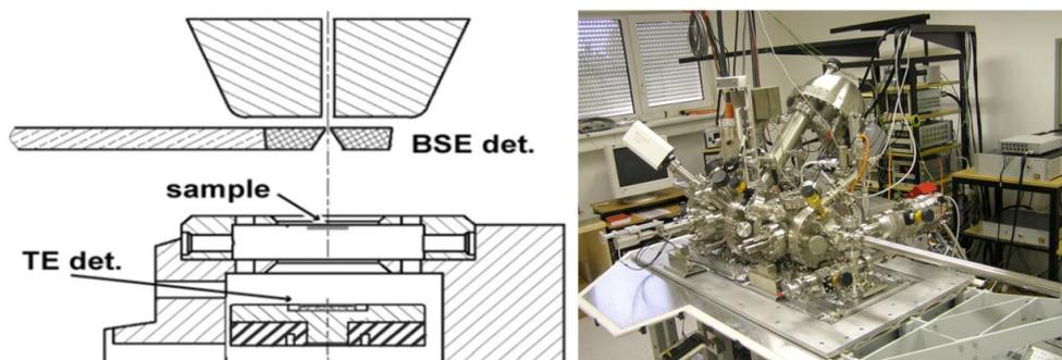
**Fig. 3** Arrangement of detectors around the sample in an ultrahigh vacuum SLEEM at ISI Brno (left); outer view of the complete device equipped with a spectrometer of Auger electrons (right).
