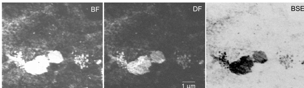
**Fig. 6.** Three simultaneously acquired image signals, namely transmitted electrons detected within polar angles of emission: BF  $\sim 0$  to 75 mrad, DF  $\sim 86$  to 366 mrad, and backscattered electrons (BSE); primary energy 4.5 keV, landing energy of electrons 500 eV, beam current 13 pA. Sample post-fixed with OsO<sub>4</sub>.
