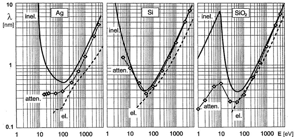
**Fig. 1** Elastic (el.) and inelastic (inel.) mean free paths and attenuation lengths (atten.) for Ag, Si and SiO<sub>2</sub>, calculated by a program simulating electron scattering in solid targets [1].
