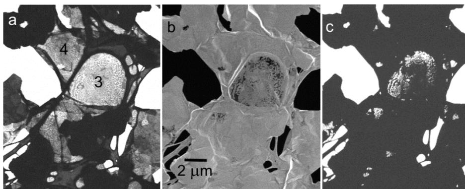
**Fig. 5.** Low energy electron micrographs of CVD graphene: transmitted electrons at 1 keV (a), backscattered electrons at 1 keV (b), and transmitted electrons at 5 eV (c) [10]. Flake no. 3 has Raman characteristics of single-layer graphene and flake no. 4 is near to these properties.
