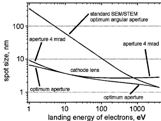
**Fig. 2** Example for a SEM/STEM with aberrations  $C_s = 7.4$  mm and  $C_c = 2.5$  mm, primary energy 4 keV, working distance 4 mm, energy spread of the beam 100 meV, gun brightness  $10^8$   $\text{Acm}^{-2}\text{sr}^{-1}$ , beam current 10  $\mu\text{A}$ , anode bore 1 mm; Barth-Kruit summation rule for confusion discs - encircled current fraction of 50%. The optimum aperture is calculated for each energy separately.
