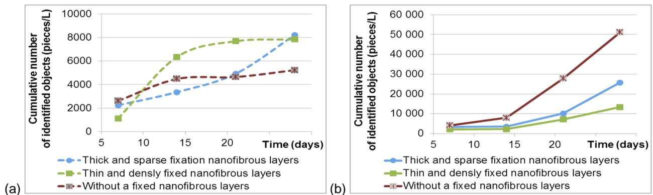
**Fig. 4** Quantification of fiber breakaway. (a) The cumulative number of all fibers present in suspension (especially larger fibers) evaluated using an optical microscope; and (b) the cumulative number of nanofibers only, evaluated using a fluorescence microscope.
