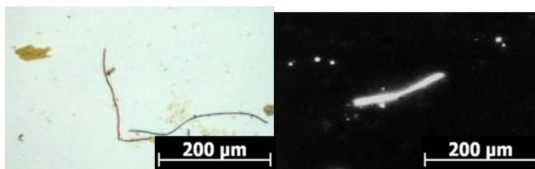
**Fig. 2** Example of image collection, surface of membrane filter scanned using an optical (left) and fluorescence (right) microscope.
