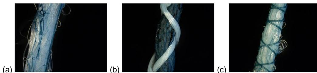
**Fig. 1** PUR nanofiber carriers. (a) with no fixation wrap, (b) with thick and sparse nanofiber fixation, and (c) with thin and dense nanofiber fixation.
