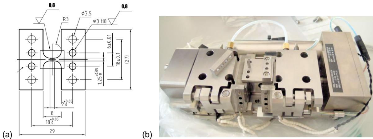
**Fig. 1** (a) Specimen geometry for in-situ tension test and (b) the Microtest™ 2000EW with EH 2000 heated grips tensile loading.
