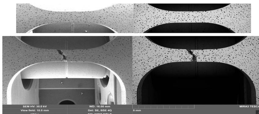
**Fig. 3** Specimen surface before (upper image) and after (lower image) tensile test.
