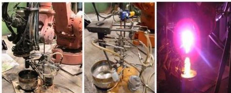
**Fig.1** Overall view of the apparatus, detail of the graphite nozzles and picture of the ongoing experiment of plasma atomization
