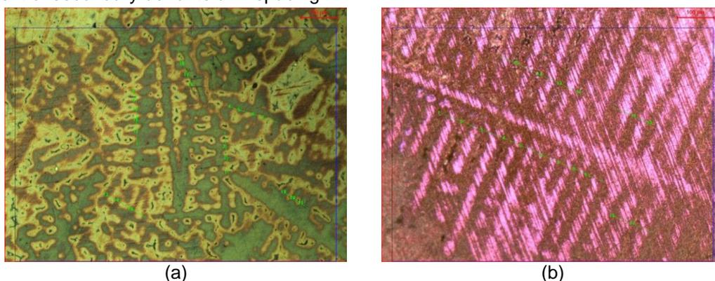
**Figure 4.** The microstructures showing the measurement of secondary dendrite arm spacing in CuSn10 alloy produced by (a) sand mold and (b) investment casting techniques.
