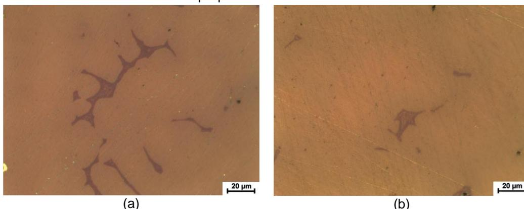
**Figure 1.** The microstructures of polished CuSn10 alloys produced by (a) sand mold and (b) investment casting technique.
