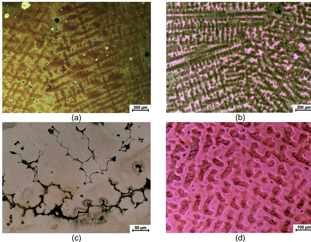
**Figure 3.** The microstructures of etched CuSn10 alloy produced by investment casting technique; (a) etched by A1 solution, in brightfield contrast, (b) etched by A3 solution, in polarization contrast, (c) etched by A2 solution, in brightfield contrast, (d) etched by A4 solution, in polarization contrast.
