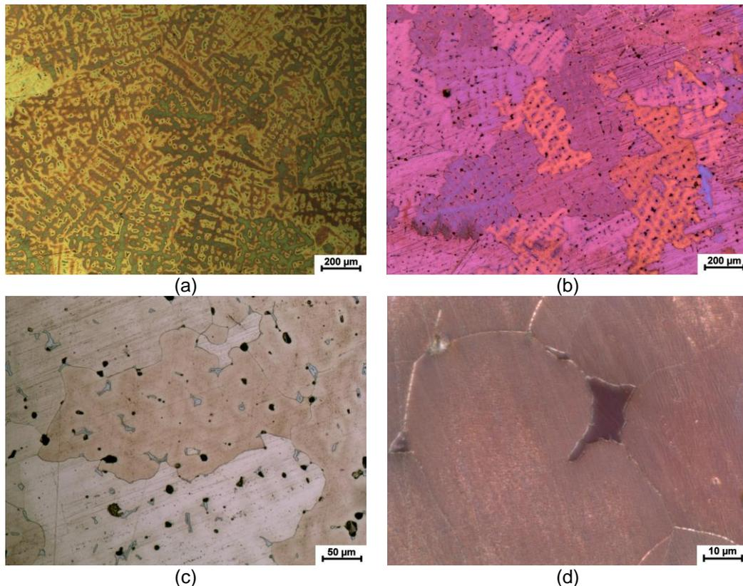
**Figure 2.** The microstructures of etched CuSn10 alloy produced by sand mold casting technique; (a) etched by A1 solution, in brightfield contrast, (b) etched by A1 solution, in polarization contrast, (c) etched by A2 solution, in brightfield contrast, (d) etched by A2 solution, in polarization contrast.
